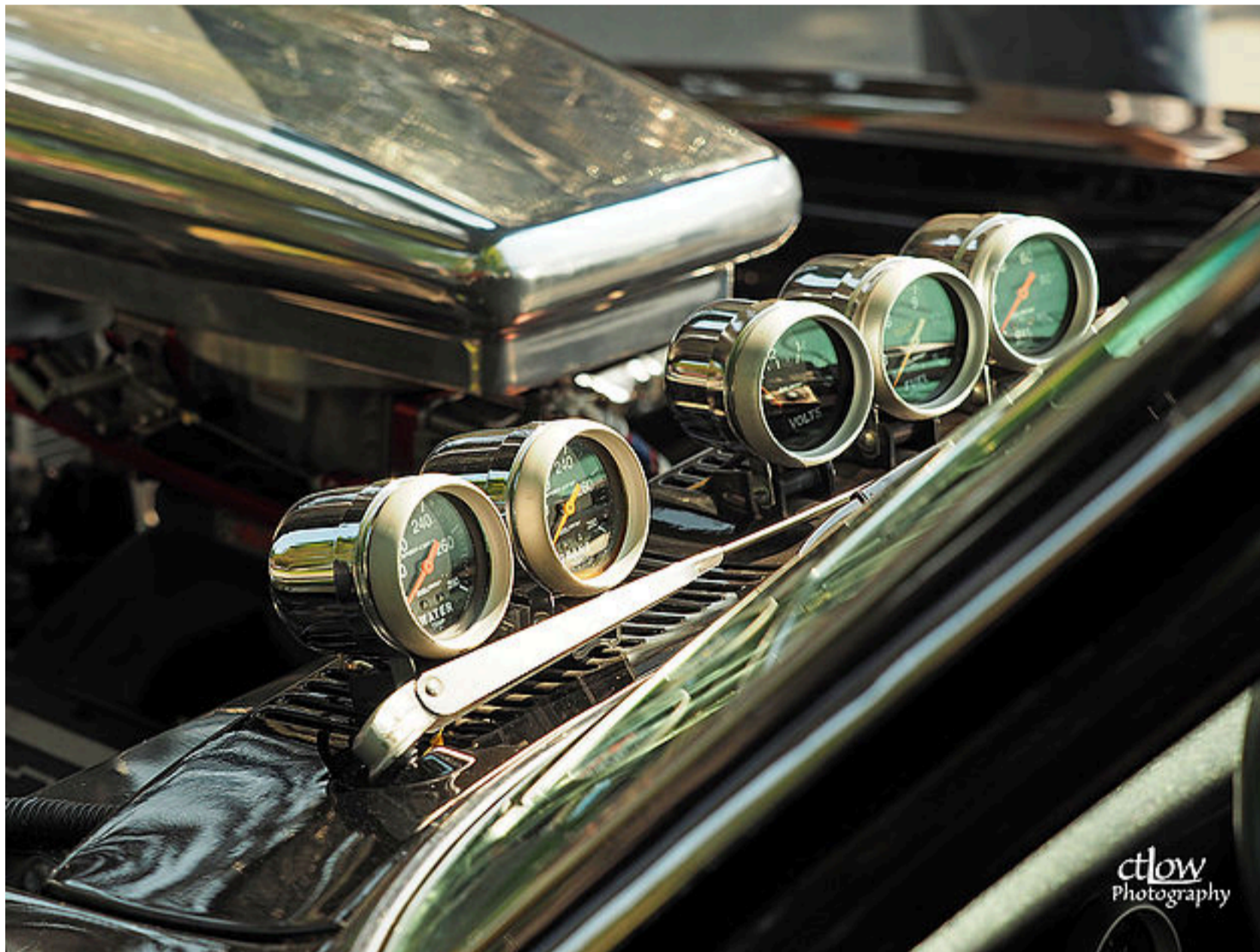
This owner apparently didn't have room on the dashboard, or didn't want to deface it, so added in all of the extra gauges, which he or she thought that the pumped-up engine deserved, on the outside of the car, just in front of the windshield wipers.
